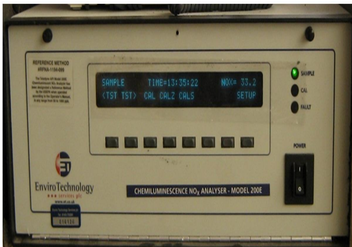
Figure 4: Automatic NO x analyser at Beresford Street Market, St Helier
