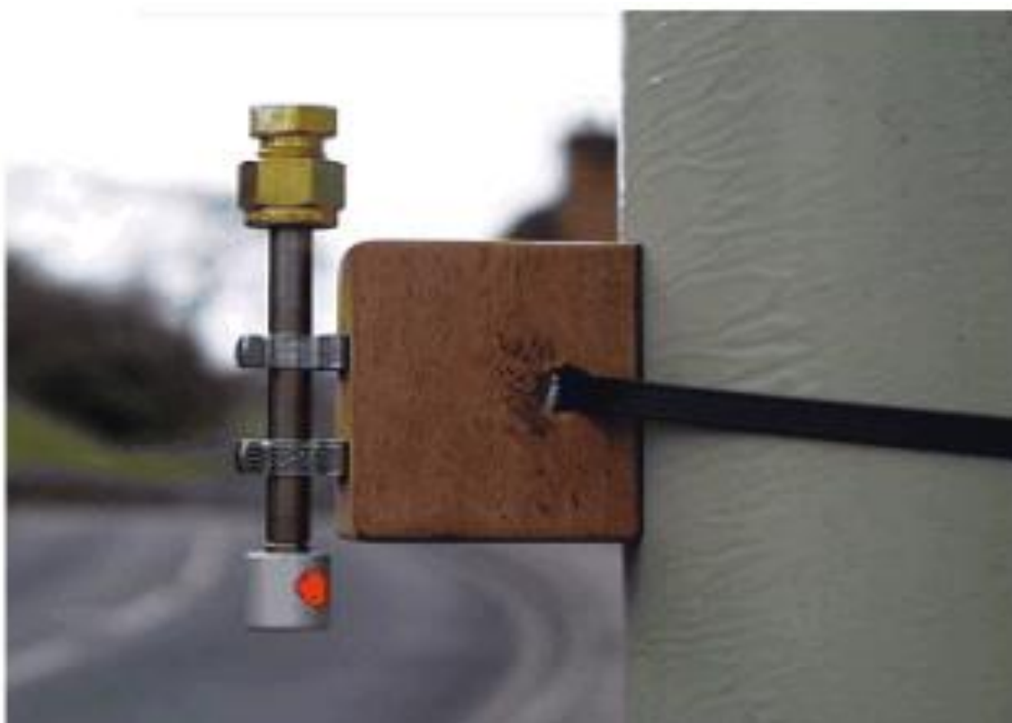
Figure 2: BTEX diffusion tube
