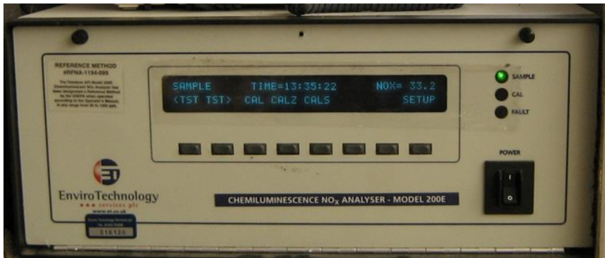
Figure 2-2 Automatic NO x analyser at Halkett Place, St Heiler
